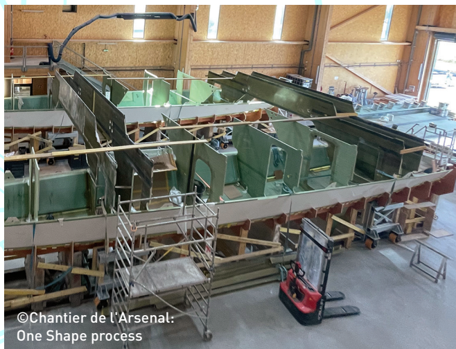
©Chantier de l'Arsenal: Assembly of ArmaPET Struct GRX sandwich panels
