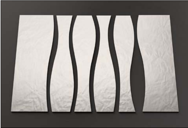
Figure 27: Primary Vapour Barrier Segment (gore) parts
