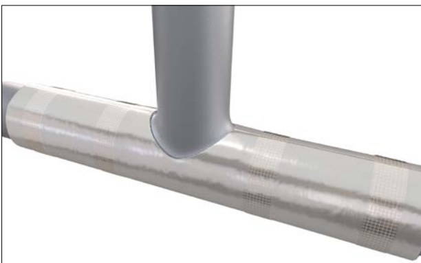
Figure 35: Securing insulation layer with filament tape
