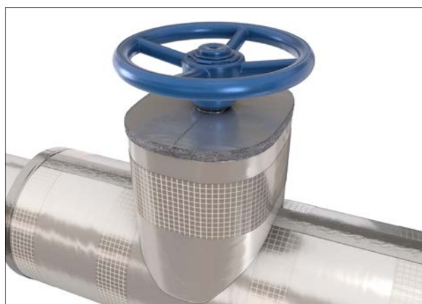
Figure 66: Insulate the top of valve spindle
