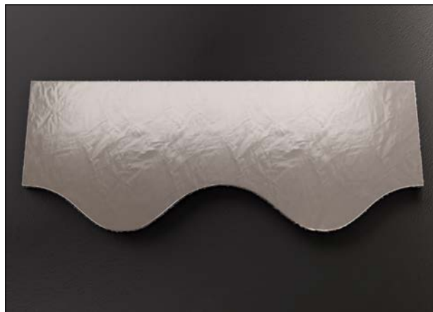
Figure 64: Fabricating the insulation for valve connection
