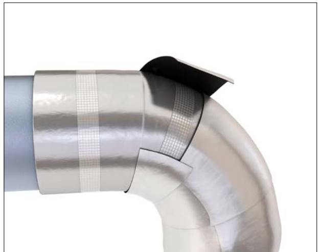
Figure 30: Application of primary vapour barrier segments
