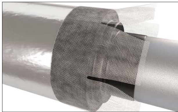
Figure 20: Feathering of flexible reinforcing membrane (50mm sections)
