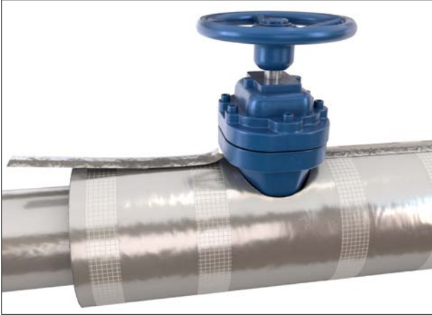
Figure 58: Application of vapour barrier tape (foil-faced butyl)
