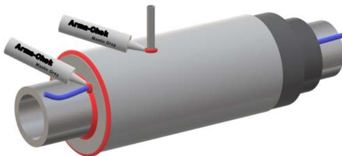
Seal penetrations with Arma-Chek Mastic (shown red for clarity)
