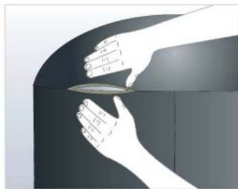
Press edges of seam together
