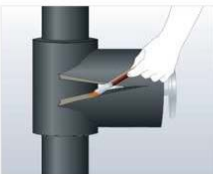
Fit T branch over actuator/stem
