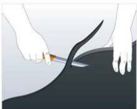
Cut T branch to fit over actuator/stem
