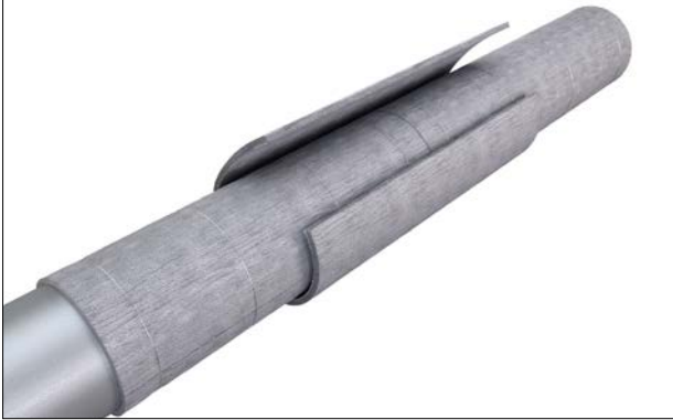
Figure 13: Staggering of next layer of ArmaGel.
