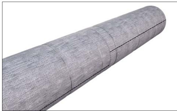
Figure 12: Rotate longitudinal seams to side
