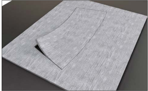
Figure 46: Cutting of reducer pattern.
