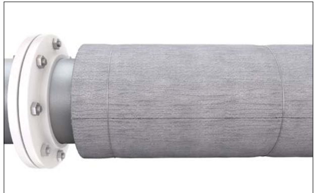
Figure 20: Termination next to a flange: bolt clearance
