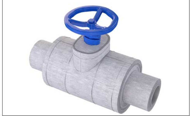
Figure 63: Installing spindle bonnet tee fitting cover.
