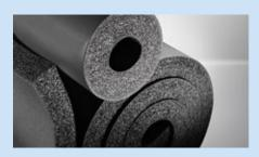
Our AF/ArmaFlex products have a completely closed-cell material structure. The vapour barrier is not restricted to a thin foil but built up – cell by cell – throughout the entire insulation thickness. The highly flexible material increases the energy efficiency of the equipment, prevents condensation, supports corrosion protection and ensures that required line temperatures are maintained. The materials are flexible and easy to install, even when installations offer limited space on board.
