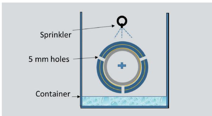
Figure 1: Test set up, showing position of drilled holes
