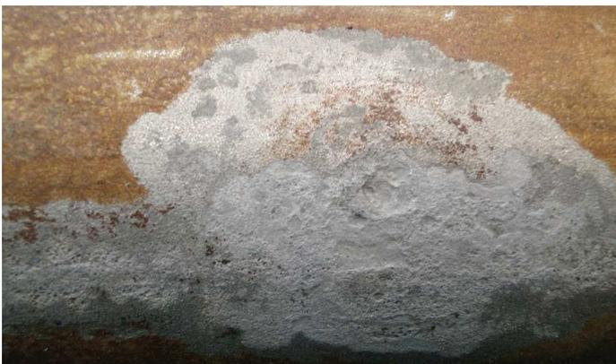
Figure 5: Close-up of the deepest area of the localised corrosion (pipe A).
