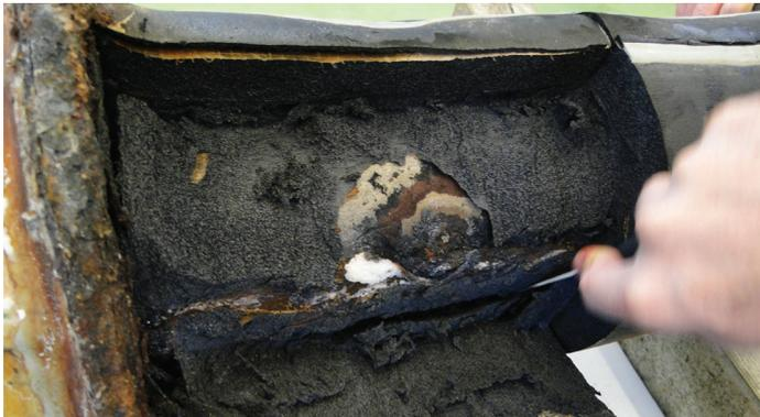
Figure 3: Insulation layers (dark grey) and adhesive layers (brownish) – corrosion localised only to the immediate areas around the holes drilled into the insulation.
