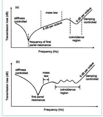
The above diagram shows the behaviour of transmission loss for a single homogeneous material (a) and a composite multimaterial sandwich construction (b)
