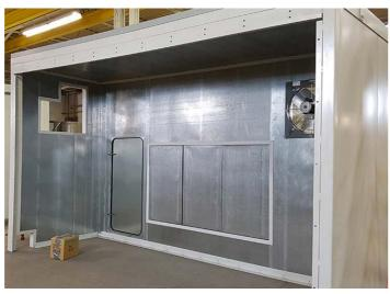
The choice of material thickness depends on the sound source characteristics/frequencies and the level of reduction required. For example, if a 50mm (2") sound absorption material was required, selecting the open cell ArmaSound RD240 option is likely to add more mass and damping to the enclosure system than may be achieved with the same thickness of mineral wool. Using the ArmaSound RD240 would therefore improve the barrier transmission loss.
