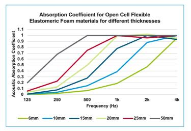
When selecting the sound absorbing porous material, it is therefore key to understand the frequencies of sound that most need to be reduced, then select a material and thickness that will best provide such a reduction.
