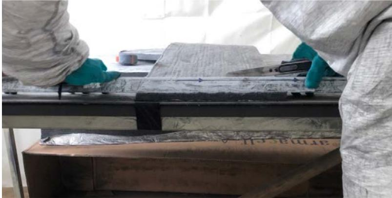
Figure 6: Cutting process using cutter and template
