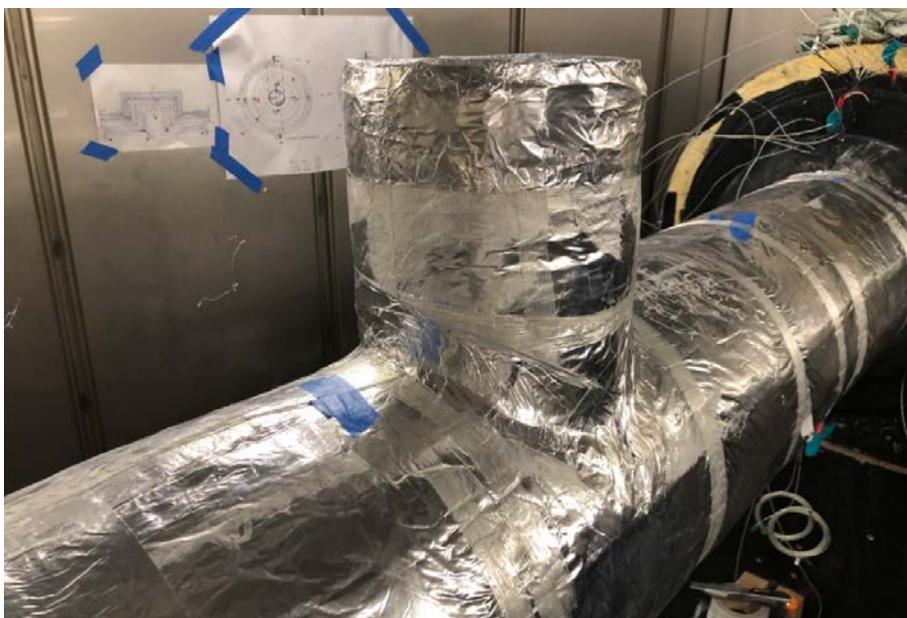
Figure 9: First insulation layer
