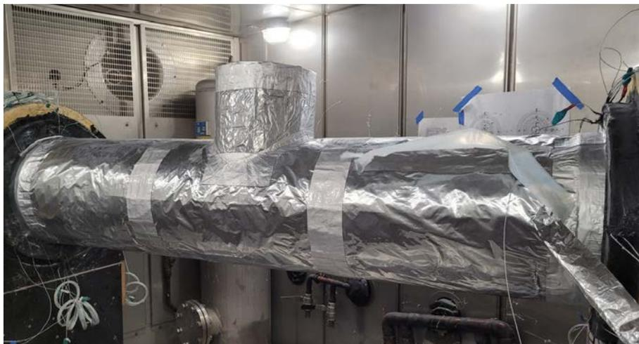
Figure 11: Installation of the vapour barrier
