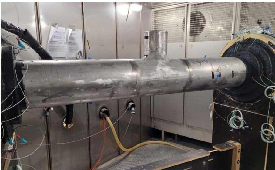
Figure 3: Test specimen in the climate chamber
