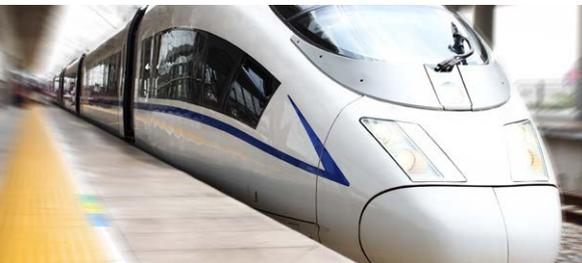
Due to its lightweight properties, recyclability, safety and long-lasting performance, ArmaPET® Struct was used for the front nose of the Chinese bullet train CRH3A.
