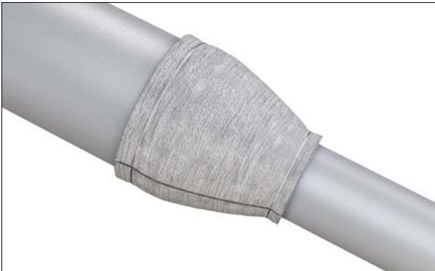
Figure 47: Securement of reducer.
