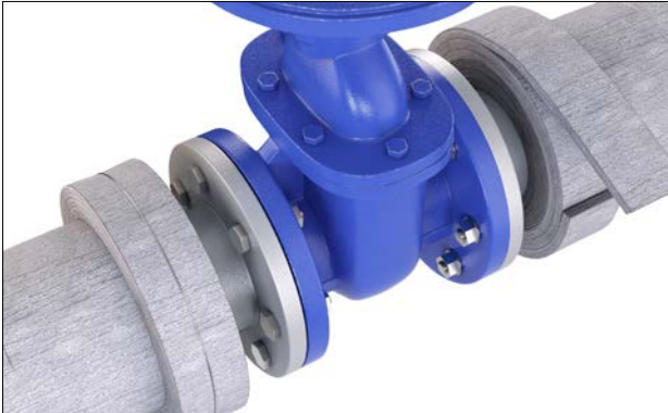
Figure 58: Preparation for valve cover.
