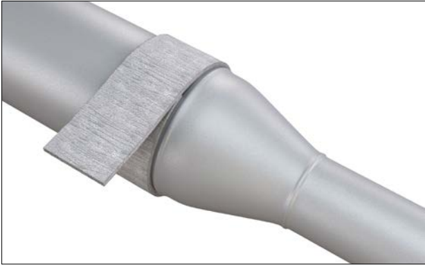
Figure 45: Measuring pipe circumference.
