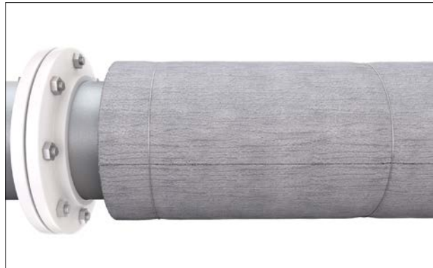
Figure 20: Termination next to a flange: bolt clearance
