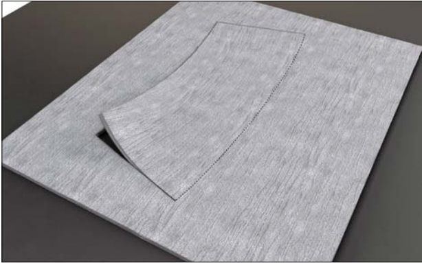
Figure 46: Cutting of reducer pattern.
