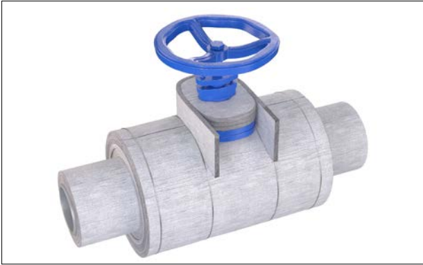
Figure 62: Fabricate spindle bonnet cap.
