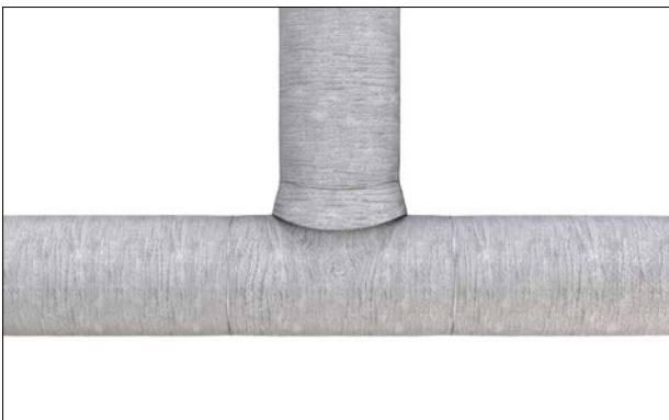
Figure 51: Installation of tee cover.
