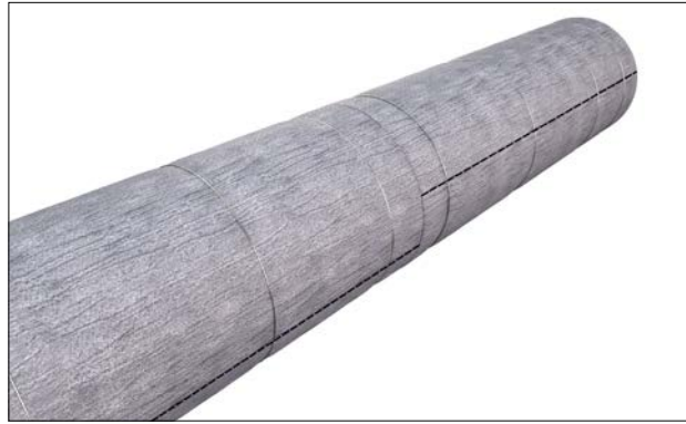
Figure 12: Rotate longitudinal seams to side
