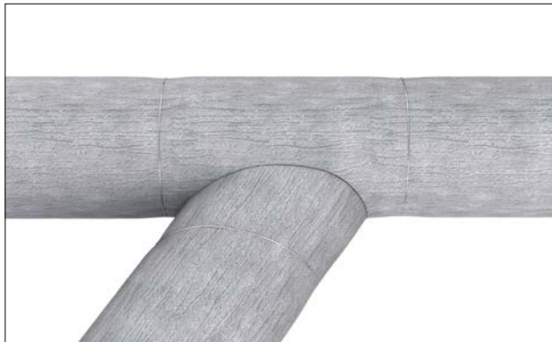
Figure 55: Completed tee cover.
